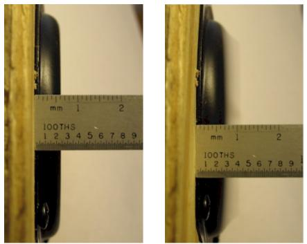
Figure 4-3: The ND90-8: excursion baseline (left) and 50 Hz at 10% 3rd harmonic distortion. (right)
