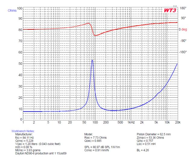
Figure 4-2: ND90 Impedance and Thiele/Small Parameters measured using the WT3 Woofer Tester
