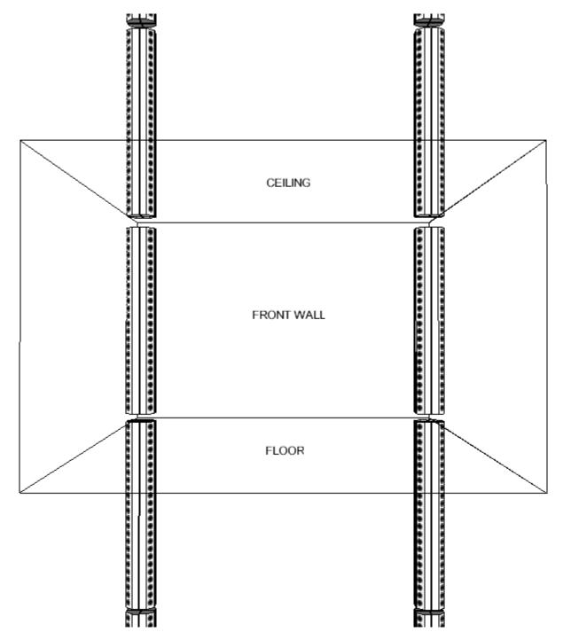
Figure 2-13: 3D View of Two Corner-Line-Array with Corner Reflections and the First Two Ceiling and Floor Reflections
