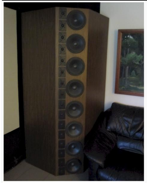
Figure A1-1: The Original Murphy-Line-Array 8/16 designed in 1980 (MLA 8/16)
