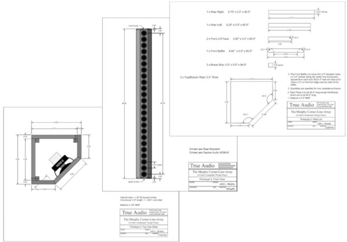
Figure 3-1: The Enclosure Drawings
