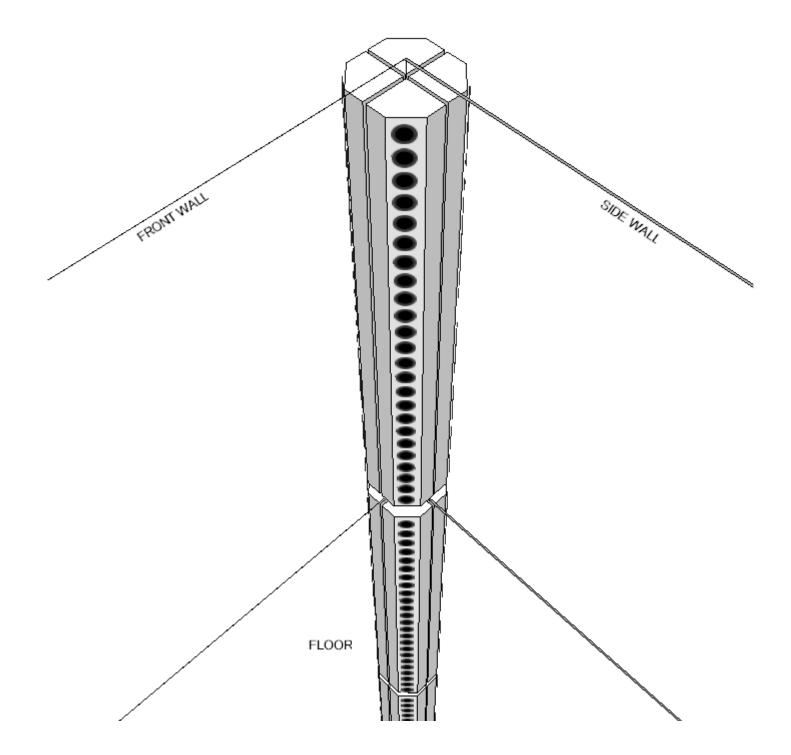
Figure 2-12: 3D View of the Corner-Line-Array with Corner and the First Two Floor Reflections
