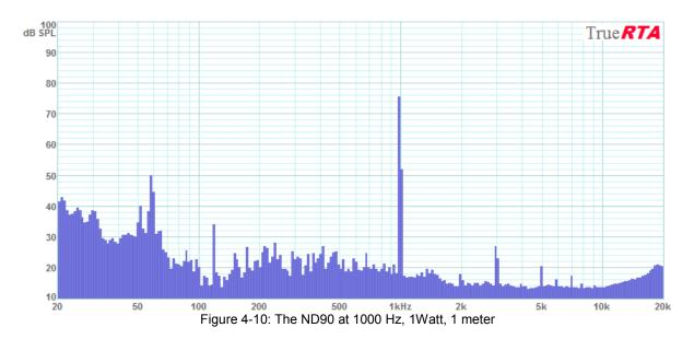
The distortion measurements for the ND90 show a driver with less than 1% harmonic distortion at the 1 Watt drive level. No other hidden distortions were evident in the course of my distortion testing. These numbers confirm what my ear had already told me: this is a nice clean little driver with no audible distortions of any type.
