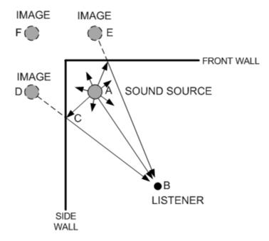
Figure 2-8: Sound Source with Multiple Reflected Images
