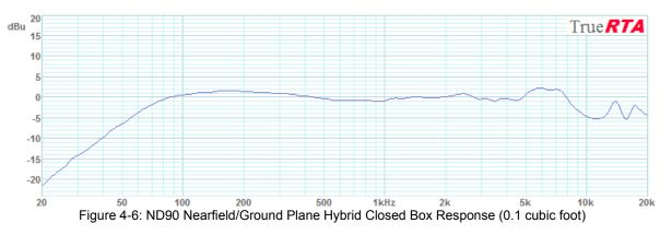
The raw response of the above closed box system is within  $\pm 2 \text{ dB}$  from about 70 Hz to 8.5 kHz. The response is within  $\pm 4 \text{ dB}$  from about 55 Hz to 20 kHz. It is the very wide frequency response range of the driver that makes this project possible.
