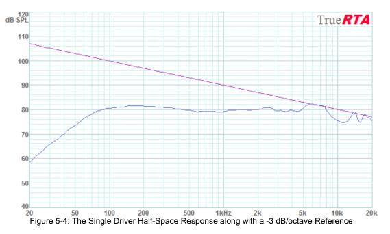
Summing the two responses shown in Figure 5-4 gives the "predicted" response for the array shown in Figure 5-5.
