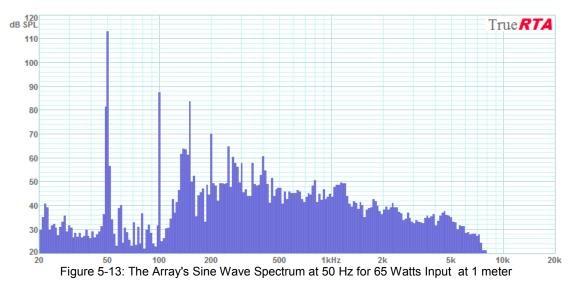
The distortion test show a speaker system capable of very high output levels with very low distortion. In all cases the distortion is dominated by the low order harmonics and is frequently dominated by the (relatively benign) 2nd harmonic. Distortion should not be a concern at even the highest sound levels...even for a single enclosure.
