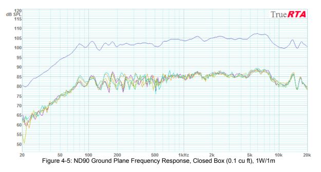
The ground plane response shown at the top of Figure 4-5 is an average of the 5 responses below with (slight) 1/6th octave smoothing. The five responses were obtained by varying the outdoor measurement geometry slightly (rotation and/or translation) between measurements in an attempt to average out variations due to reflections from the side of the house.
