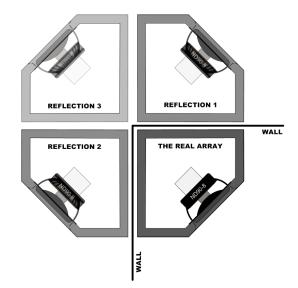
Figure A2-1: A Single Murphy Corner-Line-Array As Viewed From Above Along With Three Reflections
