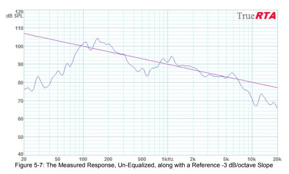
All in all the arrays achieve a frequency response much like what is expected based on the single driver measurements. The essential components required of the corrective EQ are a 3 dB upward slope (a blue filter) and EQ to extend the bass response. In practice the final EQ is best achieved by a measuring the response and adjusting the EQ a few times in succession until a sufficiently flat response is obtained.
