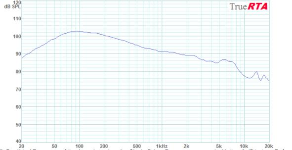
Figure 5-5: Predicted Response of the Array based on the Single Driver Response summed with the -3 dB/octave Reference
