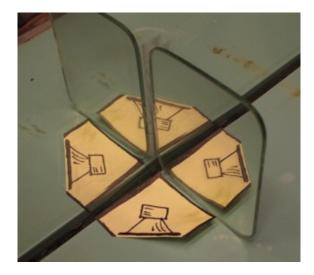
Figure 2-3: This Photograph Shows a Single Drawing of a Speaker Along With Three Reflections in Two Perpendicular Mirrors
