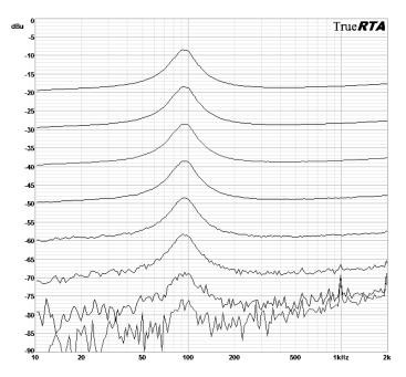
Figure 2: Impedance Response at Progressively Lower Signal Levels for a Properly Functioning Loudspeaker.
