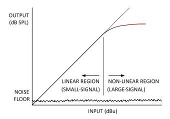
Figure 1: Small-signal versus large signal operating ranges
