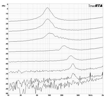
Figure 3: Impedance Response at Progressively Lower Signal Levels for a Defective Loudspeaker.
