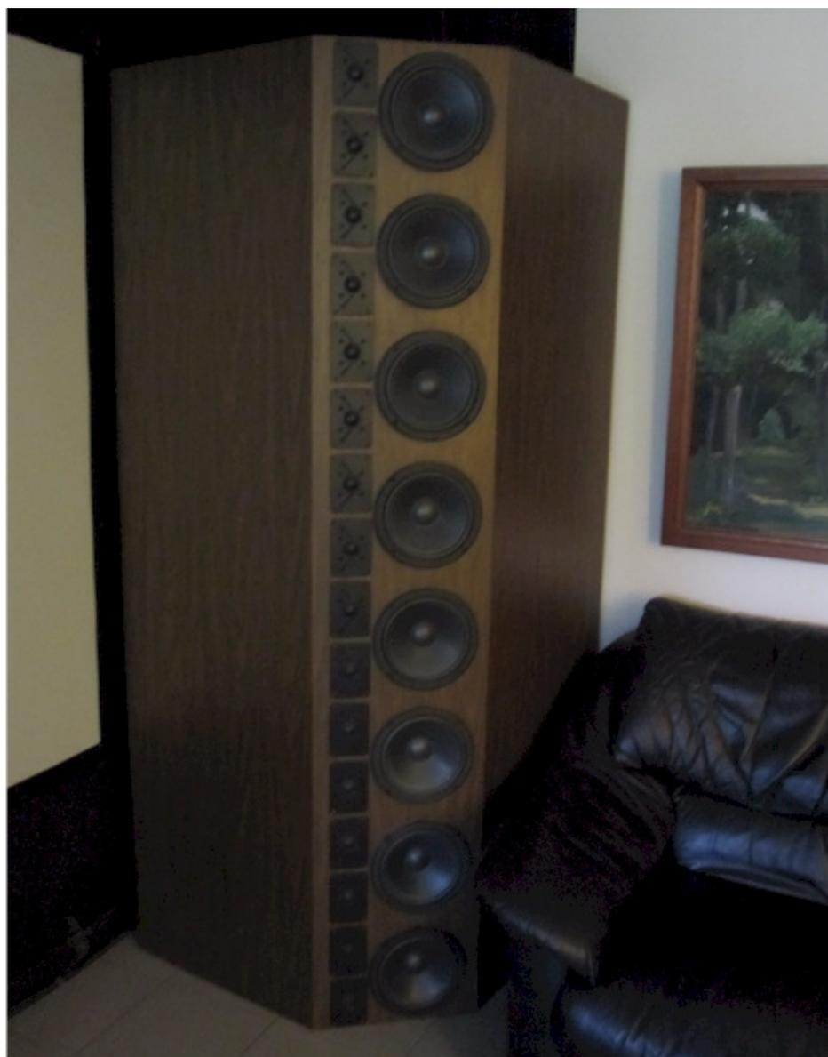
Figure A1-1: The Original Murphy-Line-Array 8/16 designed in 1980 (MLA 8/16)
